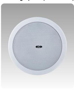
The built-in 6" speaker driver is designed of wide frequency response 110-15KHz, the multiple power taps 1.5W, 3W & 6W are helpful for different applications varies from room size and ambient noise surroundings. The metal grille and metal baffle are painted in attractive white color. Its spring clip clamp makes the easy and secure installation.
