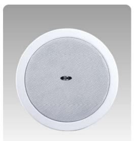
The built-in 6" speaker driver is designed of wide frequency response 110-15KHz, the multiple power taps 1.5W, 3W & 6W are helpful for different applications varies from room size and ambient noise surroundings. The metal grille, metal baffle and metal back cover are painted in attractive white color. Its spring clip clamp makes the easy and secure installation.
