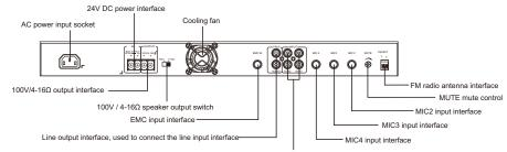
2 channel AUX input interface, used to connect AUX output interface
